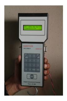
Kalpak K Test Series Force Push/Pull Gauge uses Load cells to accurately sense the Push/ Pull force on specimen under test and display it on easy to read LCD Display in lbs, Kgs or Newtons.
