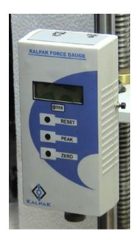
Kalpak K Test Series Force Push/Pull Gauge uses Load cells to accurately sense the Push/ Pull force on specimen under test and display it on easy to read LCD Display in lbs, Kgs Newtons or gms.
