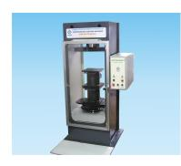
Kalpak Computerized Servo Hydraulic Compression Testing Machines are designed for testing the compression strength of cement, concrete, rocks, brick. They can also perform shear test, anti-break test and elastic modules test of concrete with special compression fixtures and measurement assembly.
